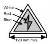
Diagram 5.4(1) - Circuit Breaker External Marking
